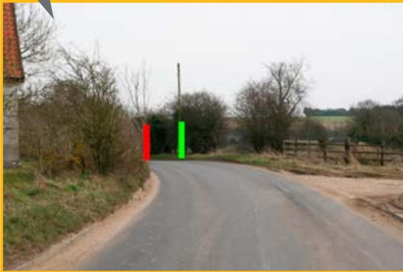
**2** The green line on the telegraph pole is used as a reference point to show the movement of the limit point.
